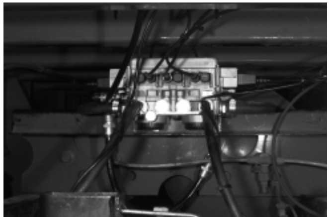
Fig. 6: EBS trailer modulator after installation
